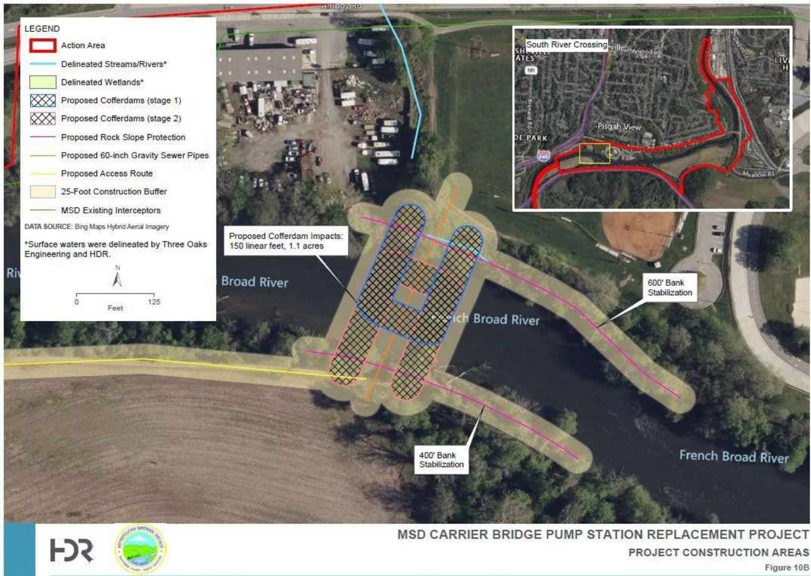
Figure 5. South River Crossing detail.
