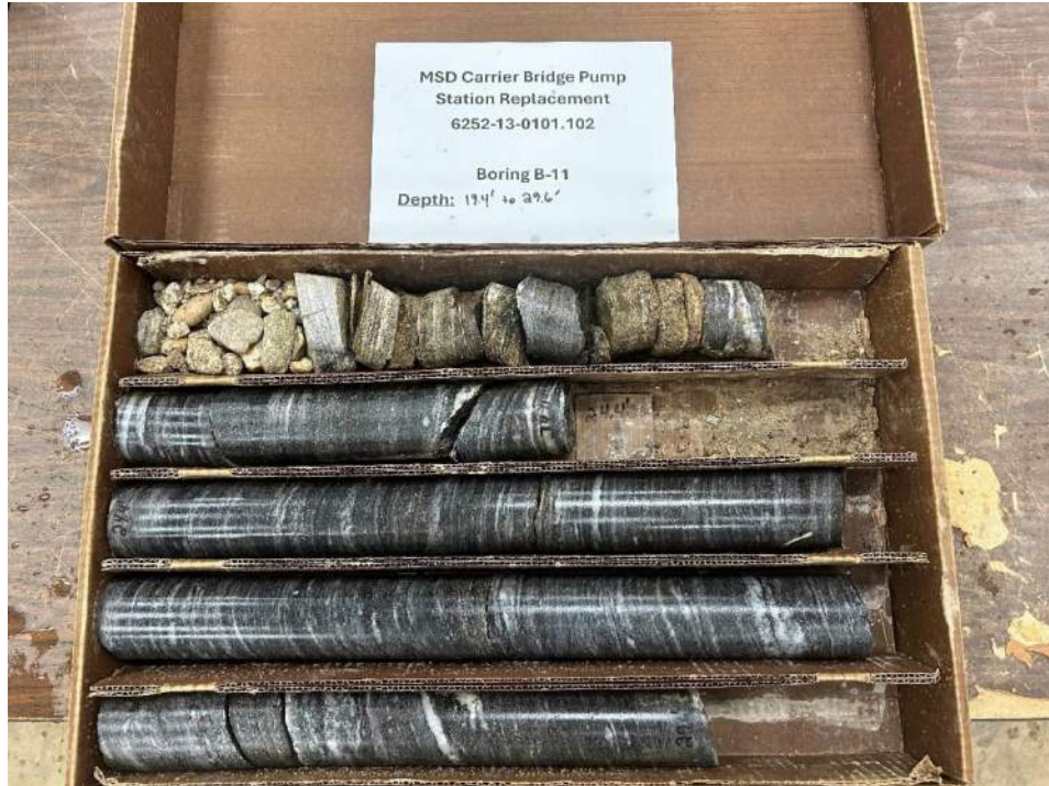
Boring Number: B-11. Core Depth: 19.4 to 29.6 Feet (going left to right and top to bottom)
