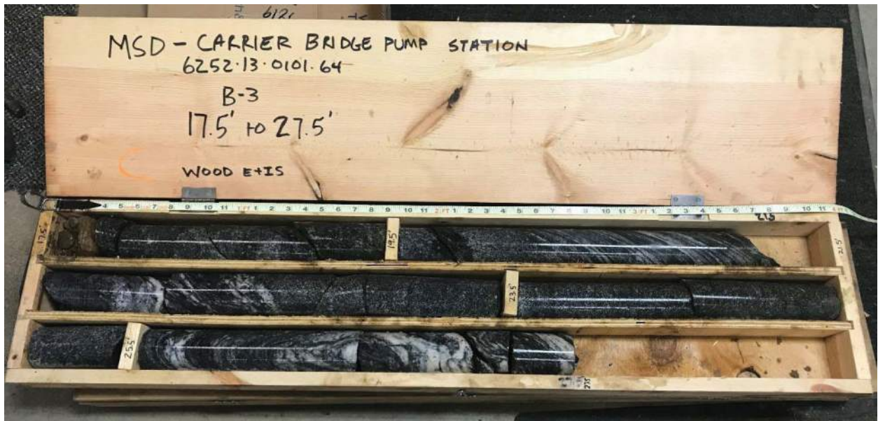
Rock core from 17.5 to 27.5 feet (going left to right and top to bottom) boring B-3
